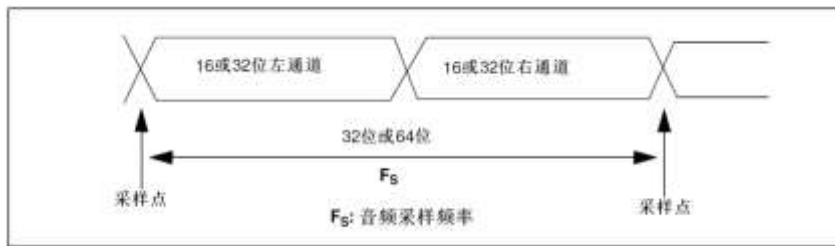
Figure 35-25 Audio Sampling Definition
